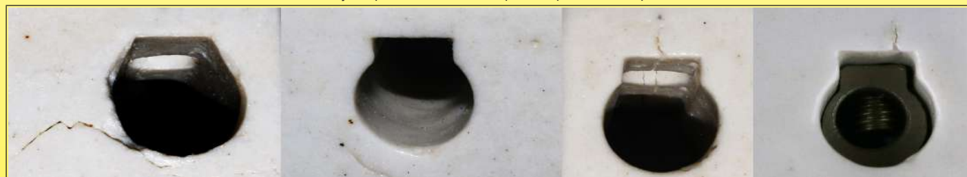
Examples of cracks on C111 porcelain
